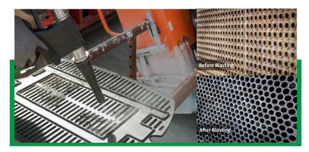
Dry ice blasting can be used on almost all surfaces, especially for mould cleaning in foundries, in tyre production, the plastic injection moulding industry and for cleaning machines and equipment include:
